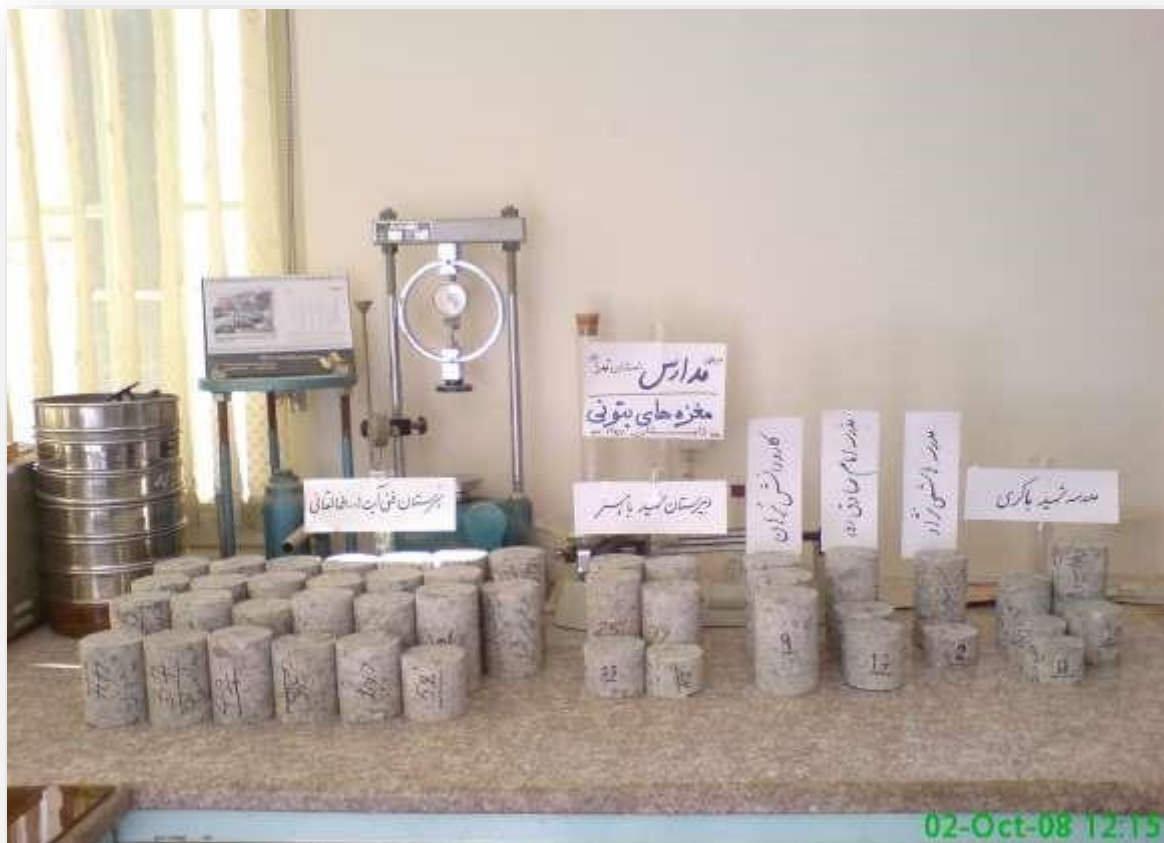
Figure-22 Concrete cores taken from schools to determine compressive strength, equipping Tehran schools (1387)
