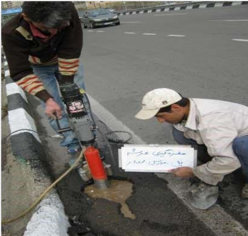
Figure-10 Core testing of Modares deck - Sadr Bridge, Technical and Engineering Consulting Organization of Tehran city (1388)
